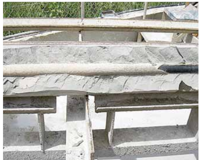
Lab testing resin mix quality – middle section of bolt
