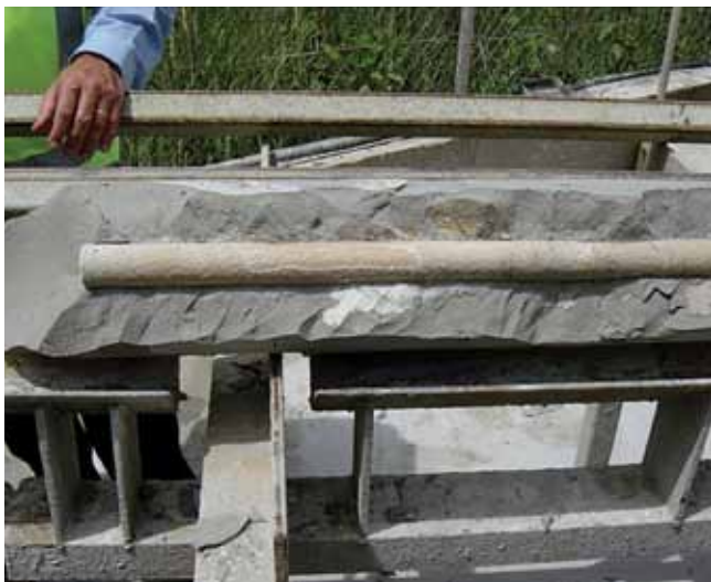
Lab testing resin mix quality – toe end of bolt
